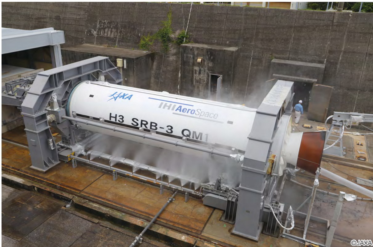
Large-size high-performance solid propellant for H3 rocket boosters
