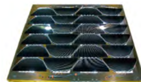
Coupon with 6" wafer-based triple-junction solar cells
