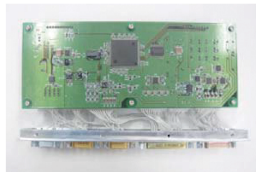
High Voltage Power Supply for MIPS
