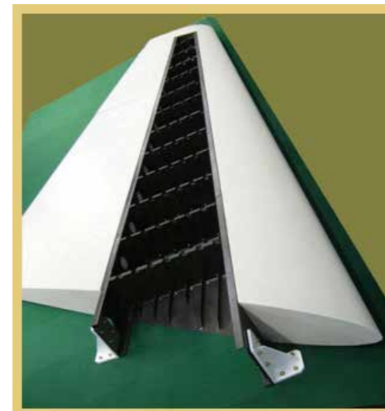
The composite main spar of the vertical stabilizer for Mitsubishi SpaceJet (actual size test component) (Mitsubishi Aircraft Corporation)
