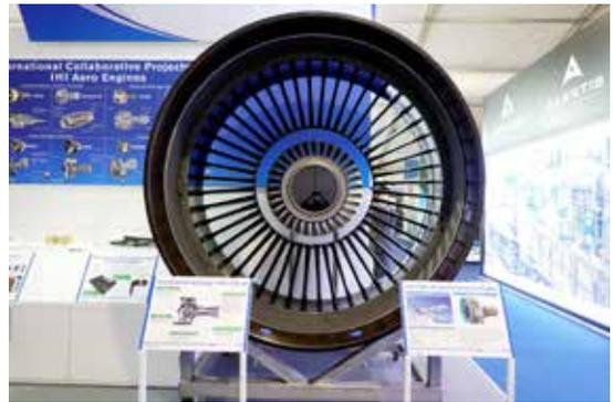
PW1100G-JM CFRP Fan Module
