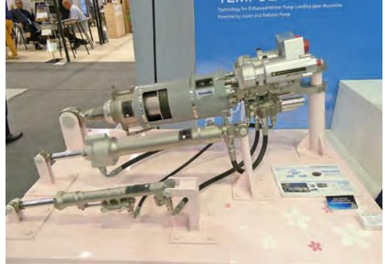
Gear EHA Assy、Door Actuator Assy、Downlock Release Actuator Assy
