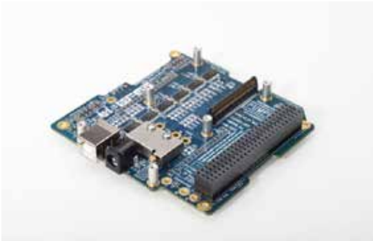
図8 PC-104規格のCubeSat基板の例 (Pumpkin社のWebページより) https://www.pumpkinspace.com/store/p49/Motherboard_Module_%28MBM%29.html
